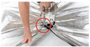
Place the casting in the centre of the canopy and insert all of the rods into the casting as shown.
