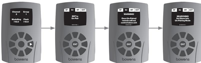
To enter un-pairing mode on the XMS press the MENU button until the display shows 'Pr' to indicate 'Pairing' mode. Use the Rotary Control to scroll through the available options until the display alternates between showing 'Pr' and 'UP' for 'Un-Pair'.
