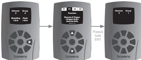
**Note: the XMSR network permits the use of up to 8 master devices (remotes in Tx mode), however to avoid setting conflicts only one of these must have the 'Remote' function enabled (see below).**
